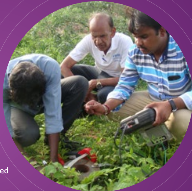
IEEE Life Member C. Satish (left) and IEEE Young Professionals Member Anvesh Kumar are testing if the earth electrode resistance is very low. This is more critical for safety in High Voltage Single Wire Earth Return distribution unlike in traditional distribution systems.
