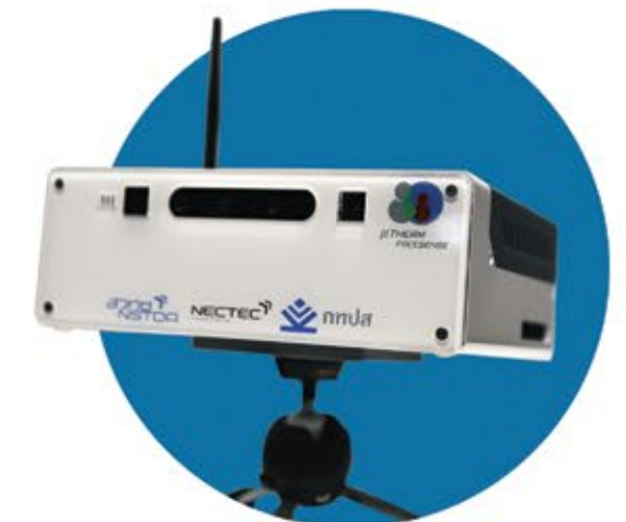
Right: Developed by researchers in Thailand, the temperature-screening system \mu Therm-FaceSense uses a visible camera, a thermal imaging camera, Lidar and facial recognition technology. Photo Credit: Komrawee Kaewmoon
