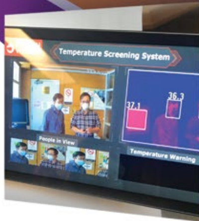
Above: The Gatekeeper camera component scans individuals, produces a visual image of each and displays their temperature. Photo Courtesy of Longan Vision
