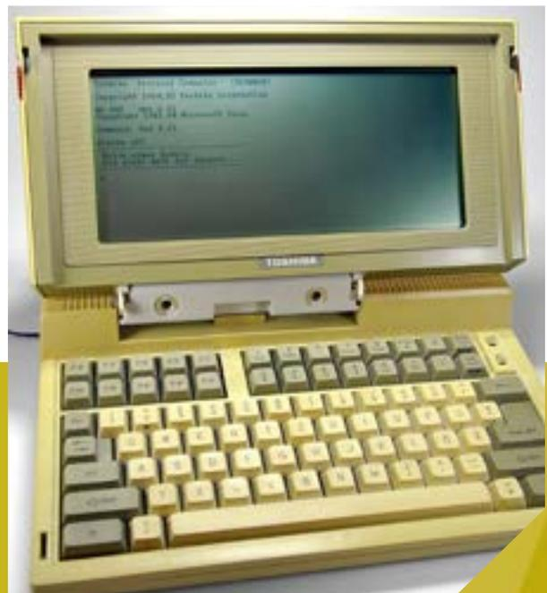
The Toshiba T1 100, an IBM PC-compatible laptop computer that shipped in 1985 made an invaluable contribution to the development of the laptop PC and portable personal computers. With the T1 100, Toshiba demonstrated the emergence and importance of true portability for PCs running packaged software. The T1 100 was a true pioneer in the development of laptop PCs, winning acceptance not only from PC experts but the business community as well.
