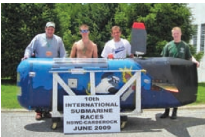
“Battlin’ Pete” from the United States Merchant Marine Academy used oscillating fins for propulsion.
