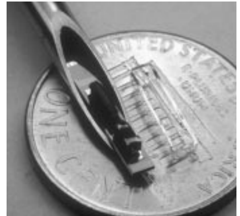
A single-channel implantable microstimulator for neuromuscular applications (developed at the University of Michigan) shown here in the bore of a 10-gauge hypodermic needle. Dr. Jeffrey Von Arx of Guidant Corporation will discuss this and other novel implantable microsystems at the 1 1/2 day interactive workshop of experts on biomedical electronics scheduled for 12–13 October in the Washington, DC area.
