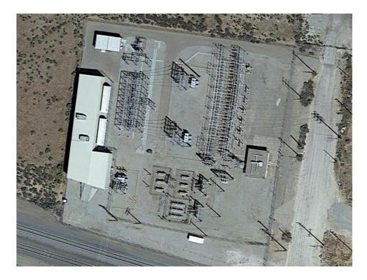
Figure 4. A monolith substation and BESS facility in Tehachapi, California. The BESS provides transmission services, system capacity, and ancillary services. (Source: Google Earth. Appeared in *IEEE Power & Energy Magazine*, vol. 15, no. 5, p. 56, Sept./Oct. 2017.)
