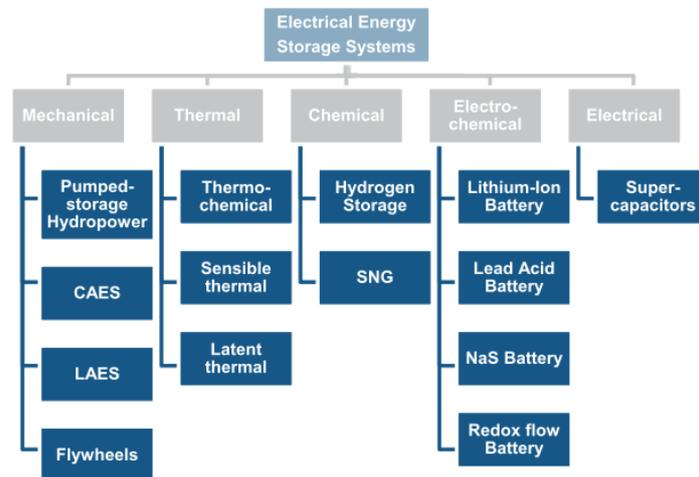
Both the amount of energy they can store as the response speed span several orders of magnitude. A correlation between these two attributes does exist. For instance, supercapacitors are able to store up to about 1 kWh to release in about 1 second, whereas pumping stations can store 10 GWh or more on daily or weekly cycles. Some technologies, such as hydrogen electro-synthesis, would be able to store even greater amounts of energy for even longer periods.
