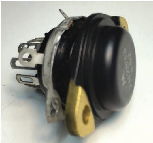
*The TO-3 and nine-pin tube socket.*
