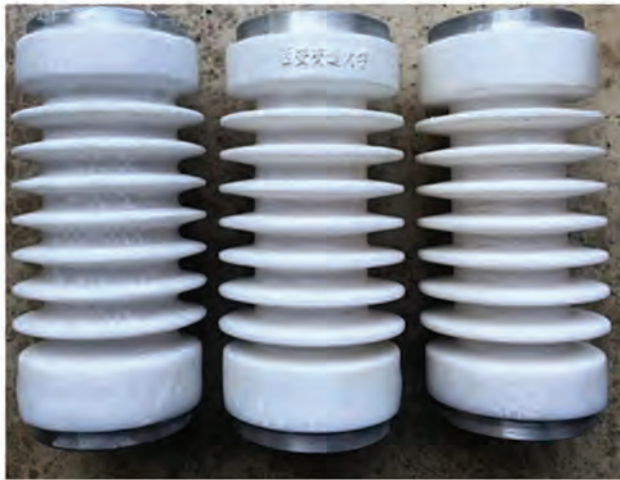
Figure 3. Fabrication and on-site commission of 10-kV dielectrically graded insulation (DGI) insulator.
