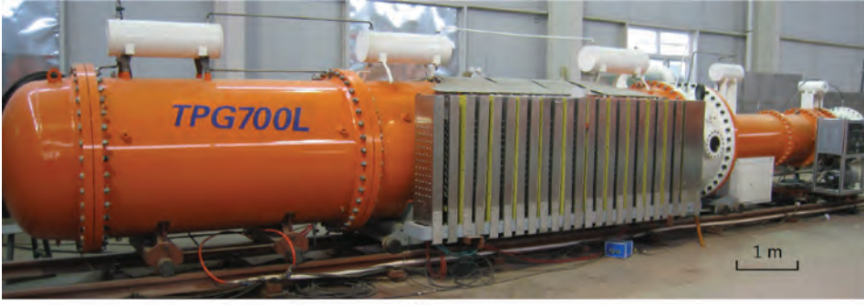
Figure 1. (a) A photo of the TPG700L pulsed power generator in the Northwest Institute of Nuclear Technology. (b) Output waveform of TPG700L.
