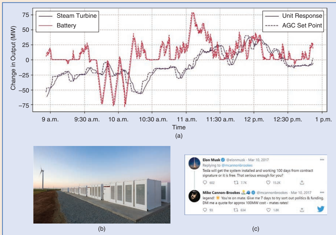
figure S2. (a) A comparison of the regulation frequency response capabilities of HPR compared to a steam turbine. (b) HPR. (c) An extract of the Twitter conversation between Mike Cannon-Brookes and Elon Musk that formed the genesis of the battery. AGC: automatic generation control. (Source: Twitter.)
